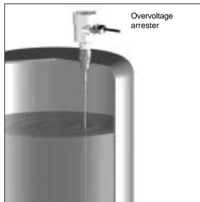
Overvoltage protection for easy mounting in the free cable entry of the sensor
